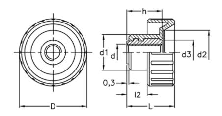
$\begin{array}{ll} d &= 32 \\ d1 &= 17 \\ d2 &= 21 \\ d3 &= 7 \\ d\ 6H = M6 \\ h &= 16 \\ L &= 22.0 \\ l2 &= 9.0 \end{array}$
